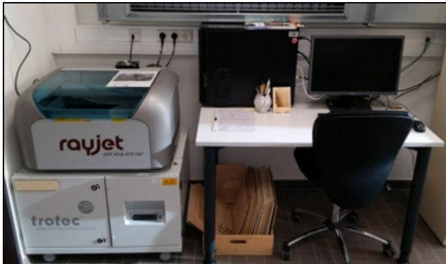
The Rayjet 50 is a CO 2 Laser engraver/cutter
