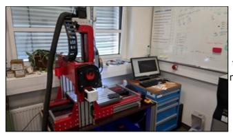
The Rising Phenix is a fixed gantry CNC portal milling machine
