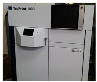
The Trump TruPrint 1000 is a LMF (LASER Metall Fusion) system for direct printing of metallic materials.
