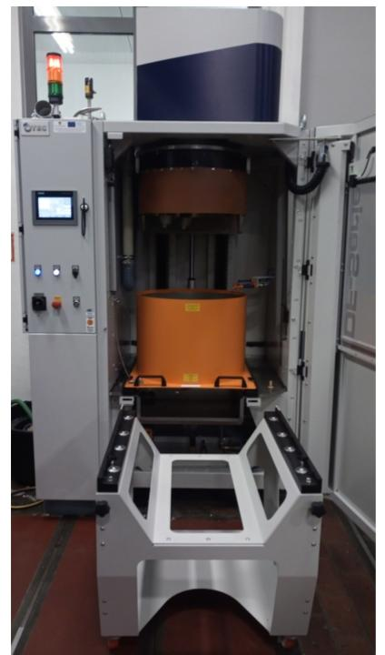
Container volume Maximum immersion depth Maximum workpiece diameter Editing media 80 l 250 mm 210 mm Ceramics, plastic, corn granules
