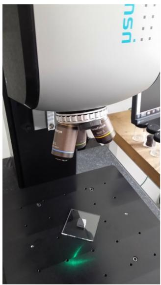
The Nanofokus µsurf expert is a confocal microscope with which surface structures can be visualized.
